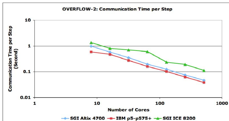
Fig. 1: Communication time for OVERFLOW-2 for Altix, POWER5+, and ICE systems.
